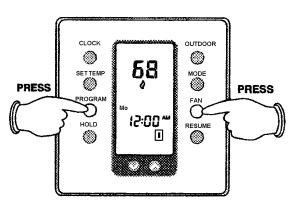
To activate the progressive recovery mode simultaneously press the **PROGRAM** and **FAN** buttons. A small thermostat icon, " , will appear under the clock. Once in this mode proceed with programming your thermostat remembering to use exact times for each event time change.
